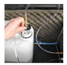
Remove the Priming Tube from its resealable bag and, holding the open end into the barrel, insert the plastic connector into the 'fluid out' port on the machine. A small amount of fluid may begin to immediately move through the tube. The connector requires a firm push until it clicks into place.
