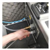
The next steps involve moving fluid into and through the machine so it is vital that the open end of the Priming Tube is held into the barrel <u>at</u> <u>all times</u> to avoid spills and waste!
